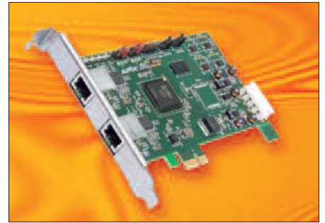
Figure 3: congatec PCI Express APIX expansion card
