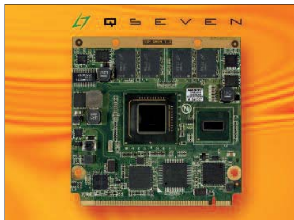
Figure 1. conga-QA – an easily integrated, small size PC module based on the Intel Atom processor
