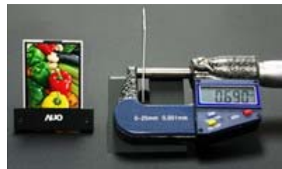
AUO ultra-thin 1.9-inch mobile device TFT-LCD with a thickness of 0.69mm
