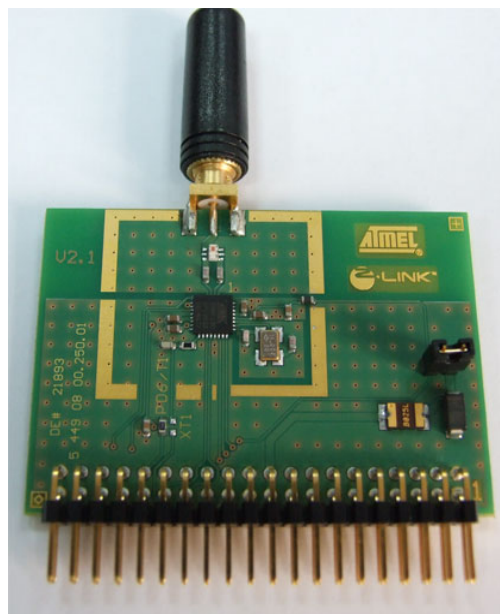
Figure 1. The RZ502 Board with SMA stab antenna
