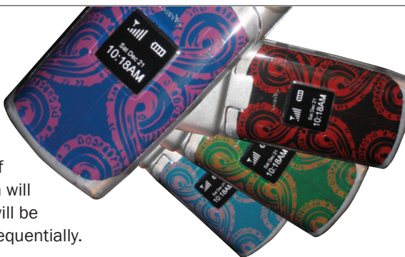
[Figure 5] Development stage: patterned and curved Reflex Electronic Skins applied to a cellular phone. (actual photos)
