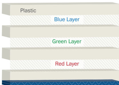
[Figure 2] Cross section of an electronic skin where inside surfaces are coated with conducting polymers.
