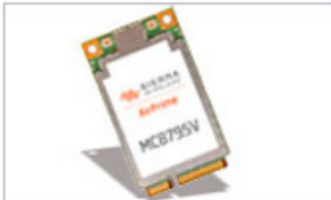
AirPrime™ MC8795V Intelligent Embedded Module Quad-band HSPA PCI Express embedded module
