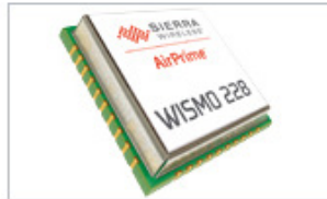
AirPrime™ WISMO228 Intelligent Embedded Module Quad-band GSM/GPRS entry-level module for industrial wireless M2M
