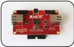
XC-3 LED Tile Controller Card, 5V Power Supply, XTAG Connector USB Cable
